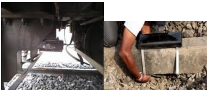
RFID Reader beneath Loco
