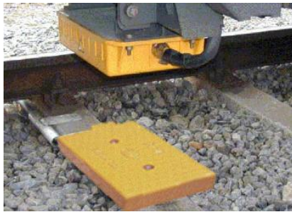
Figure 2-1 shows balise produced by YooKyung Control (Inc).
