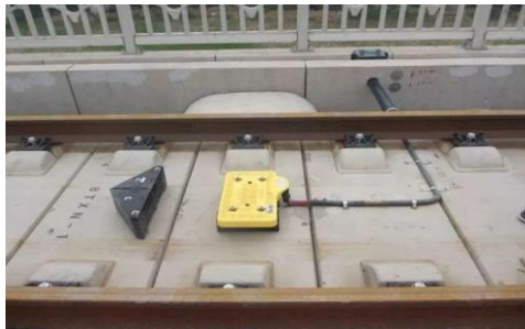
Figure 3-1 Balise used in Chinese high-speed railways
